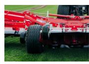
The chassis tyres are 15% wider than the previous model distributing weight evenly across the turf.
